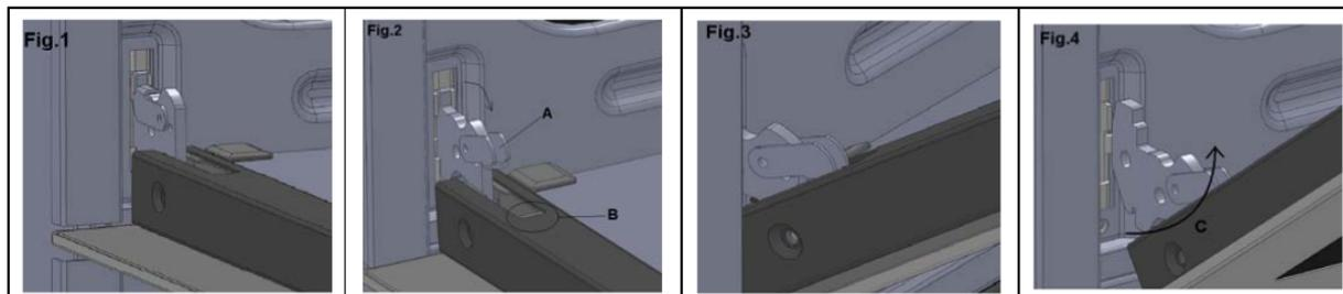
Put the door to one side, resting it on a soft surface. Clean the glass with an appropriate cleaner. Dry thoroughly. To refit the door, repeat the steps above in reverse order.
