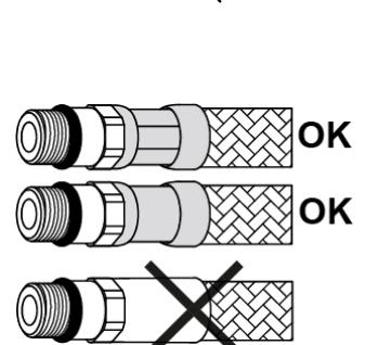
Before assembling the hose to the product ensure the hose ferrule has been crimped (as highlighted) on both ends of the hose after the braided hose sleeve.
