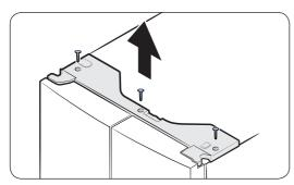
**1.** With the door closed, use a **Phillips** screwdriver to remove 3 screws on the top cover with the wire connectors.
