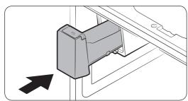
**3.** Remove the remaining ice cubes and put the ice bucket back into place.
