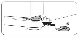
**2.** Insert a suitable-sized **snap ring (A)** between the door and the hinge as shown.
