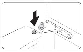
**2.** While pressing down the hinge shaft of the door, reinsert the door into the middle hinge.
