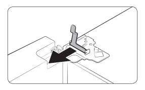
**2.** Disconnect the two connectors on the left door. The position of the connectors differs with the model.
