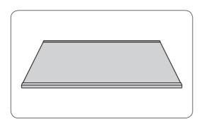
To secure more room in the freezer or the CoolSelect+ (FlexZone) compartment, remove the middle drawer of the freezer or the CoolSelect+ (FlexZone) compartment, and then insert the freezer shelf between the middle and bottom drawers.
