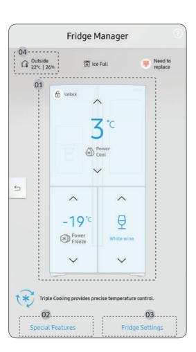
The Fridge Manager is a graphical representation of your refrigerator. The top half represents the refrigerator compartment, the bottom left the freezer compartment, and the bottom right the Cool Select+. The temperature or mode settings for each are displayed over each section. Fridge Manager At a Glance
