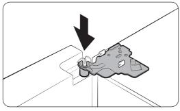
**2.** Put the top hinge into its position, and then insert into the top hole of the door.
