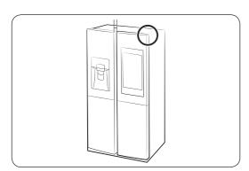
Door gaps can be corrected using the gap bolt on the top right corner of the refrigerator.
