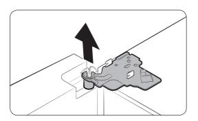
**6.** Open the door by 90 degrees. While holding the door, remove the top hinge.
