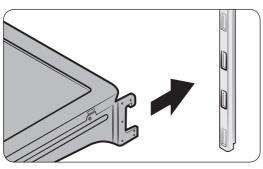
To reinsert, lower the rear side of the shelf and insert into the shelf hooks.
