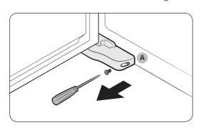
**1.** With the freezer door open, use a Phillips screwdriver to remove the screw holding the **cover (A)** of the adjustable leg.
