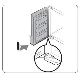
**1.** Insert the freezer door into the bottom hinge while pushing the freezer door in the arrow direction.
