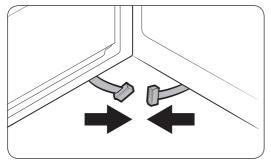
**3.** With the door open, connect the bottom connectors in the arrow directions.
