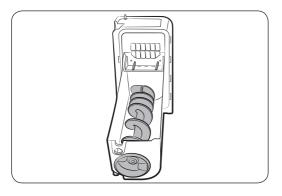
If the ice bucket is not firmly inserted, turn the ice screw by 90 degrees and try again.
