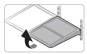
To remove a shelf, fully open the corresponding door. Hold the front of the shelf, and then gently lift up and slide out.
