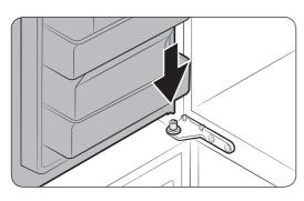
**1.** While holding the door open by more than 90 degrees, reinsert it into the middle hinge.
