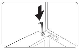
3. Locate the hinge shaft. While holding the door with one hand, use a flat-head screwdriver or wrench to press down the shaft. Make sure to hold the door to prevent the door from falling.
