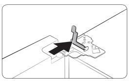
**3.** Insert the clamp in the arrow direction.
