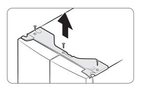
1. With the door closed, use a Phillips screwdriver to remove the screws (x3) from the top cover. Pull up and remove the top cover with the connectors.
