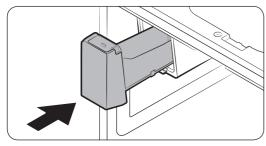
**3.** When done, put the bucket back into position. If the bucket does not fit in, turn the helix screw by 90 degrees and try again.
