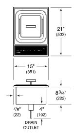
$\ensuremath{\text{NOTE:}}$  Dimensions in parenthesis are in millimeters unless otherwise specified
