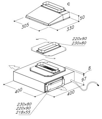
Offset nozzle piece (**C**) can be fitted to the top of the motor to allow it to be fitted closer to the rear of the cabinet - offsetting the motor to the downdraft - which can be used in setup option 1 (see page 4).
