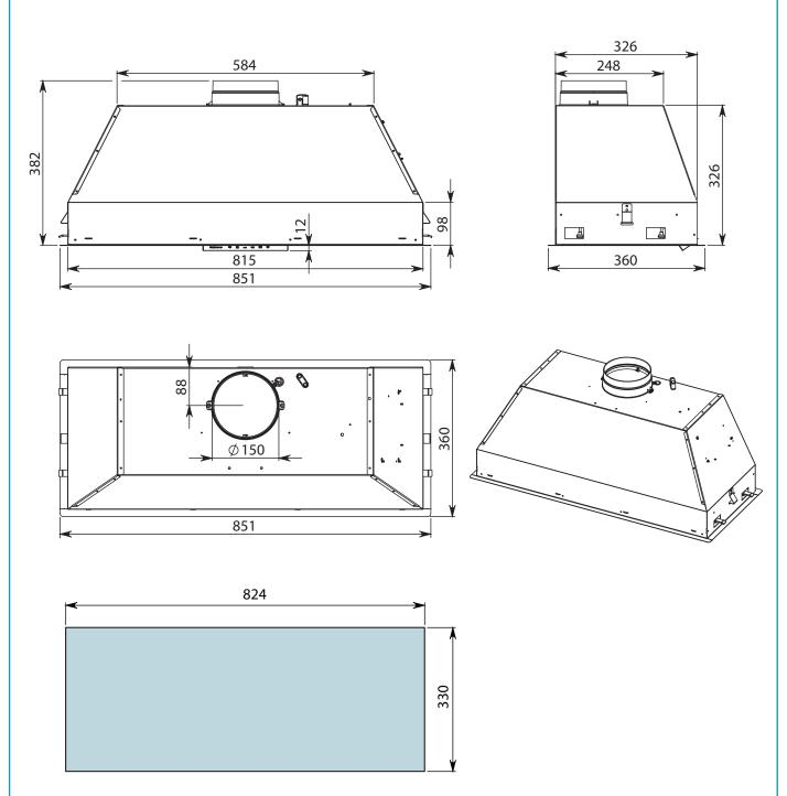
EN - HOLE MEASUREMENTS FOR INSTALLATION
