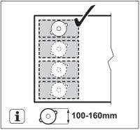
Place the cookware with the bottom diameter larger than 160 mm centrally between two sections.
