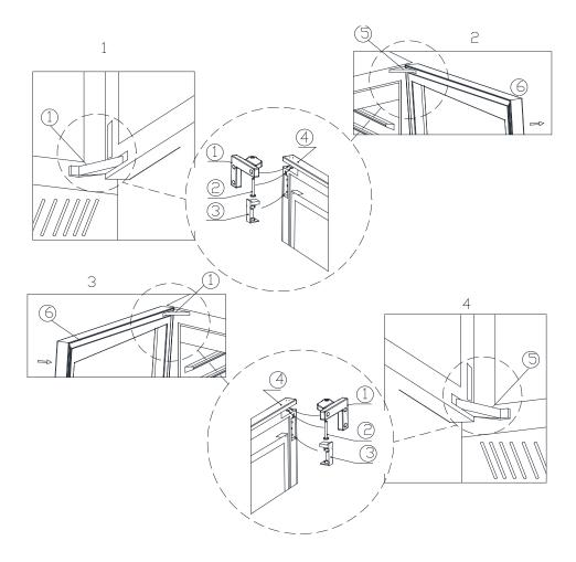
①Upper hinge ②Hinge shaft ③Hinge buckle ④Upper hinge ⑤Lower hinge ⑥Glass door 1. As shown in Figure 1, use a flat-blade screwdriver to open the upper hinge buckle ③ to see the hinge shaft ②, and then use a flat-blade screwdriver to pry the hinge shaft ② and take it out. Then unscrew
