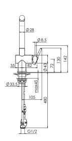
**PLEASE NOTE:** Large and heavy taps should ideally be mounted directly through the solid benchtop or fully supported from underneath. For all other swivel taps, we recommend the use of the Franke Tap Support Arm to provide additional support. Please ensure all Franke tapware is installed at a pressure of no greater than 500 kPa in accordance with AS/NZS3500 and insist that your plumber flushes all of the water supply lines before installing tapware. Failure to do so may void warranty.
