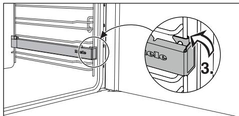
■ Then secure the FlexiClip telescopic runner to the lower rail of the shelf level as illustrated (3).
