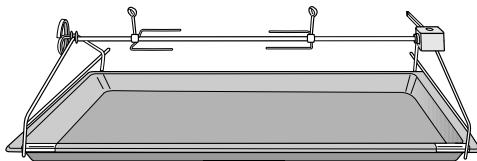
The rotisserie can be used to grill thicker items such as rolled meat and poultry. Food is grilled evenly on all sides as it rotates.
