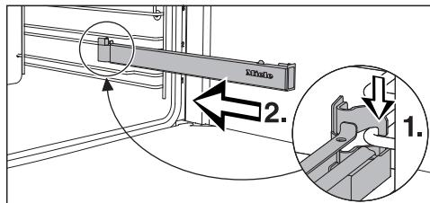
■ Hook the FlexiClip telescopic runner onto the lower rail of a shelf level at the front (1.) and push it along the rail into the oven interior (2.).
