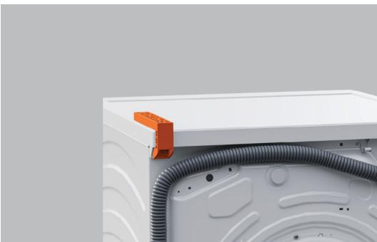
2. Fit Brackets onto the rear of the washer.
