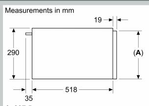
**A:** 287.5 mm Ovens with appliance height of 595 mm can be installed above the warming drawer without an intermediate floor
