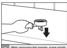
After removing the tamper, some grinds may stick to the side of the filter basket. Tap the portafilter gently on the table to jostle loose grinds onto the tamped coffee disc. Do not tap too hard, or the tamped coffee will dislodge or fracture.
