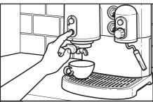
Place one or two espresso cups on the drip plate under the spouts of the portafilter. Press the Espresso button, and espresso will start to flow into the cups.
