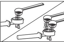
Remove the portafilter from the brew head by moving the handle to the left. Place one level measure of ground coffee (or a paper coffee pod) in the small filter basket, or two measures of ground coffee in the large filter basket. Be sure to use a fine espresso-style grind for your coffee.
