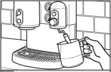
With the Steam dial closed, adjust the frothing arm so it's in a comfortable working position, and submerge the tip of the frothing nozzle just below the surface of the milk in the frothing pitcher.
