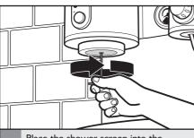
Place the shower screen into the brew head with the smooth side facing down, and attach with the shower screen screw. Turn the screw clockwise until snug.
