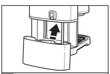
Place the reservoir back into the 3 Espresso Machine, making sure the water tubes are placed inside the reservoir. The ribs on the bottom of the reservoir fit into the grooves on the base of the machine.
