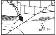
The frothing arm and nozzle should always be cleaned after milk is frothed. Remove the frothing sleeve from the frothing nozzle by pulling it downward. The frothing sleeve can be washed in warm, soapy water. Make sure any openings in the sleeve are free of residue.
