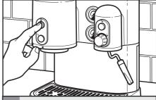
Press and hold the On/Off power button until the ON indicator lights up. The dual boilers will begin heating, and the Espresso and Hot Water functions will begin to operate.
