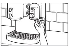
Wipe the frothing arm and nozzle with a clean damp cloth. Do not use an abrasive scouring pad.
