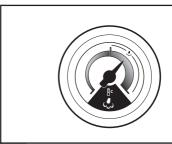
Wait until the Espresso Machine has reached operating temperature; it may take approximately 6 minutes. When the frothing boiler temperature gauge needle climbs into the "ready" zone, the Espresso Machine is ready to froth.
