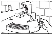
Slowly open the Steam dial by turning it counter-clockwise. The further the Steam dial is rotated, the greater volume of steam will be released. Tilt the pitcher to one side to create a whirling motion in the milk, keeping the tip of the frothing nozzle about 6.4 mm below the milk's surface.
