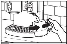
Keep the pitcher tilted to maintain a whirling motion in the milk. Steam the milk until it's between 60 and 73.9°C. (At these temperatures, the pitcher will be very warm to the touch.)
