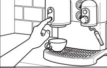
After removing the portafilter, place a cup under the brew head and press the Espresso button for a second or two. This cleans the shower screen and flushes out any coffee oils and grounds that have migrated into the brew head.
