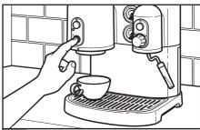
Press the Espresso button to activate the water pump and fill the brewing boiler with water. After a few seconds, water will flow from the brew head. When the cup is full, press the Espresso button again to stop the water pump. The brewing boiler is now ready for use.
