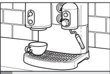
Place a coffee cup underneath the brew head. Do not attach the portafilter to the brew head.
