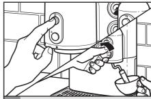
Plug into a grounded outlet and turn on the Espresso Machine; let the boilers reach operating temperature. Point the frothing arm into an empty cup and momentarily open the steam dial to run steam through the frothing nozzle. This will clean the nozzle tip.
