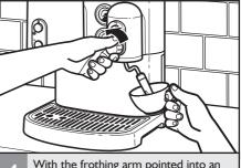
With the frothing arm pointed into an empty cup, open the Steam dial for a moment to purge excess water from the line. To open the Steam dial, turn it slowly counter-clockwise. To close the Steam dial, rotate it clockwise until it stops.
