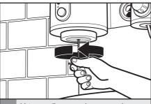
Using an allen wrench, remove the screw at the center of the shower screen by turning it counter-clockwise.
