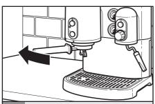
The Espresso Machine is equipped with a 3-way solenoid valve that instantly releases pressure in the brew group when the water pump is switched off, so the portafilter can be removed immediately after brewing. Remove the portafilter by moving the handle to the left. Knock the used coffee grounds out of the filter basket into a waste container.
