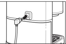
Insert the end of the electrical cord without prongs into the cord receptacle in the back of the Espresso Machine. Plug the other end of the cord into a grounded outlet.
