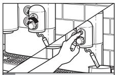
6 Slowly open the Steam dial by turning it counter-clockwise; press and hold the Hot Water button to activate the water pump and fill the frothing boiler. After a few seconds, water will start flowing from the nozzle.
