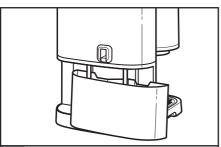
Lift the reservoir slightly, then remove by pulling the bottom of the reservoir from the Espresso Machine.
