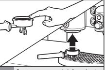
Sweep any excess grinds from the rim of the portafilter, and insert into the brew head.
