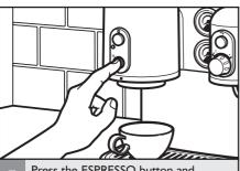
Press the ESPRESSO button and dispense cleaning agent through brew head for 15 seconds; press the ESPRESSO button again to shut off.
