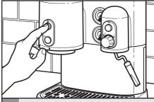
Wait 20 minutes, then repeat steps 4–7. Every 20 minutes, keep repeating steps 4–7 until nearly all the solution in the reservoir has been run through the Espresso Machine. Do not allow the reservoir to run completely dry.
