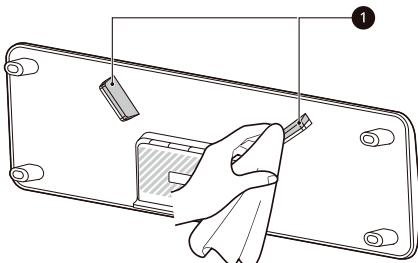
3 When cleaning is completed, reinstall the lint filter cover on top of the lint filter correctly.
