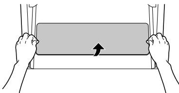
2 Remove the aroma filter ① from the back of the lint filter cover ②.
