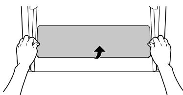
2 Wipe the mirror surface on the back of the lint filter cover with a soft dry towel.
