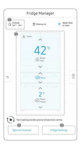
The Fridge Manager is a graphical representation of your refrigerator. The top half represents the refrigerator compartment, the bottom left the freezer compartment, and the bottom right the Cool Select+. The temperature or mode settings for each are displayed over each
