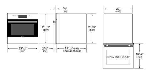
$\ensuremath{\text{NOTE:}}$  Dimensions in parenthesis are in millimeters unless otherwise specified
