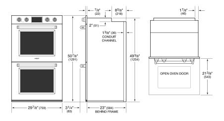
$\ensuremath{\text{NOTE:}}$  Dimensions in parenthesis are in millimeters unless otherwise specified
