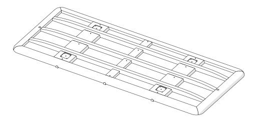
b) One at a time, turn each leg upside down, position it into the relevant rebate in the underside of the tabletop subframe, and secure with  $4 \times M6 \times 30$  Countersunk screws tightened with an Allen key.
