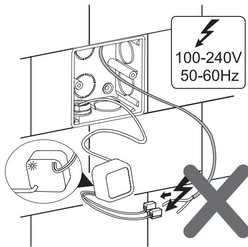
The size of cable should be  $1.0-2.5\text{mm}^2$  and the wire connector should be connected firmly.
