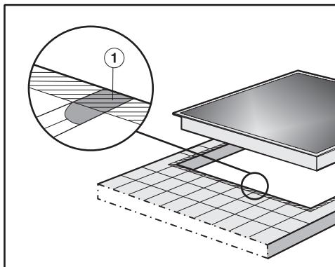
Grout lines ① and the hatched area underneath the cooktop frame must be smooth and even. If they are not, the cooktop will not sit flush with the worktop and the sealing strip underneath the cooktop will not provide a good seal between the cooktop and the worktop.
