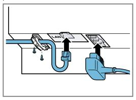
3. Connect the LAN cable to a network connection.
