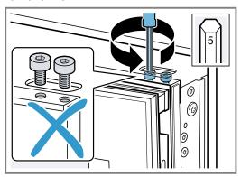
4. Adjust the appliance door using the side screw; to do this, open the appliance door and then close it again if necessary.
