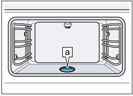
If you remove the drain filter a before the cleaning programme is started, the cooking compartment will not be clean.
