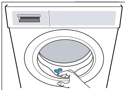
3. Clean the outside and the inside of the rubber gasket with a damp cloth and wipe dry.
