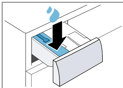
5. Add washing powder containing oxygen bleach to the manual dosing compartment.
