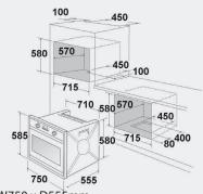
$\begin{array}{lll} \mbox{Product Dimensions:} & \mbox{H585} \times \mbox{W750} \times \mbox{D555mm} \\ \mbox{Cut-out size (proudmount):} & \mbox{H580} \times \mbox{W715} \times \mbox{D570mm} \\ \mbox{Cut-out size (flushmount):} & \mbox{H588} \times \mbox{W753} \times \mbox{D570mm} \\ \end{array}$
