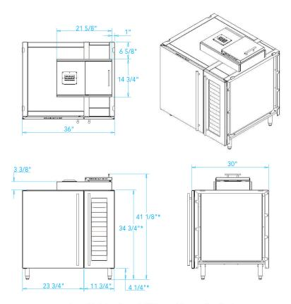
\*overall height adjusts +/- 3/4" on stainless steel leveling legs
