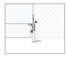
The Lateral Connection Kit (KCLIT/KCLIH/KCLMT/ KCLMH) is supplied on all models (except in the unit with stainless steel sides) and consists of a connection element (A) and a aluminium
