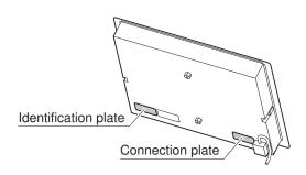
► Affix the second identification plate (supplied) in an accessible position behind the front of the fitted cabinet beneath the appliance.
