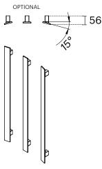
Heated rail is supplied with offset adapter which allows for the above 3 installation options. Left, right or flat facing.
