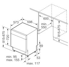
measurements in mm
