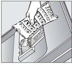
Add dishwasher salt only until the reservoir is full or until water runs out of the opening. The salt reservoir holds approx. 1 kg of salt, depending on the brand used.
