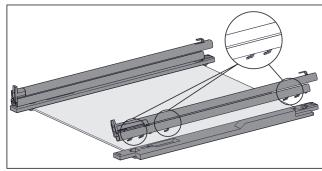
Fig. 116 Glass shelf with rails and retaining parts
