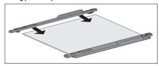
Fig. 118 Glass shelf with retaining part
