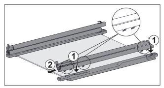
Fig. 120 Glass shelf with rails and retaining parts Install rail with damping mechanism:
