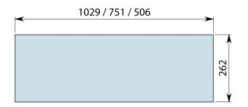
HOLE MEASUREMENTS FOR INSTALLATION
