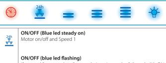
If pressed for more than 3 seconds, it activates the 24h cycle (1h ON -> 3h OFF -> 1h ON)
