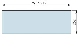
HOLE MEASUREMENTS FOR INSTALLATION
