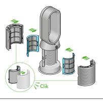
The air purifier fan heater with the filter covers open showing a HEPA plus carbon filter located in the filter covers and a catalytic filter. Arrows demonstrate that the catalytic filter is fitted directly to the base of the machine and the filter covers will need to be assembled onto the base of the machine.
