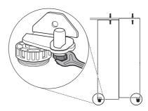
Open the door and use the spanner 10 to loosen the keeper nut by turning it to the left.
