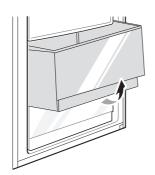
**2** Press on the hook inside the top compartment, and then take out the Air Filter.
