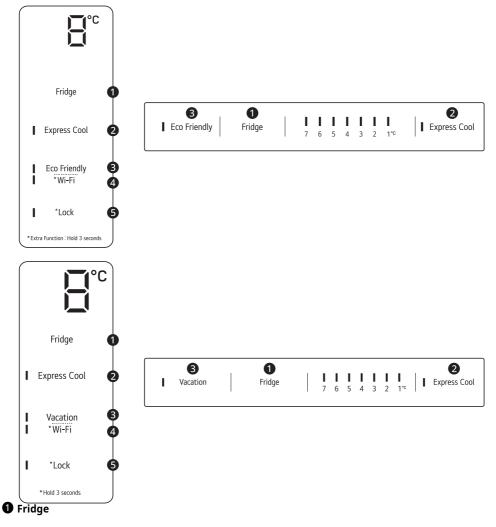
Press this button repeatedly to select a desired temperature between 1 °C and 7 °C.
