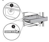
2 Tilt the drawer and remove it by pulling it out.
