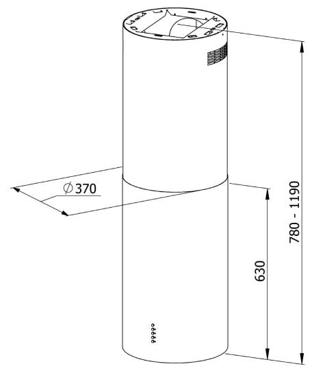
Model: X370GV Island Hood Size: 37cm diametre Power standard: 10 Amp plug Ducting size: 150mm
