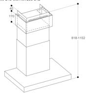
$^{\star}$  Suitable for ceiling heights from 2.45 m to 2.75 m; Specifications refer to the distance of 1.60 m from the floor to the lower edge of the hood.
