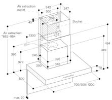
\* Suitable for ceiling heights from 2.25 m to 2.55 m; Specifications refer to the distance of 1.60 m from the floor to the lower edge of the hood.
