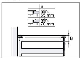
**4.** Mark the unit cut-out in accordance with the installation diagram.
