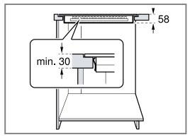
3. Maintain the minimum clearance from the upper edge of the worktop to the upper edge of a drawer installed below it.
