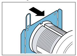
**8.** On the rear of the control knob, tighten the retaining nut using the installation tool provided.
