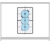
For a diameter over 13 cm, position the cookware on one of the three positions as shown in the illustration.
