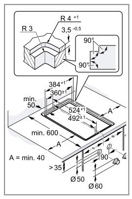
5. Ensure that the angle of the cut surface to the worktop is  $90^{\circ}$ .
