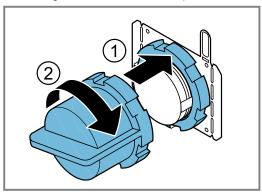
9. Align the control knob precisely in the zero setting.
