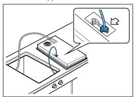
2. Ensure that the plug engages in the socket.
