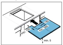
**8.** Observe the clearance between the intermediate floor and the worktop.
