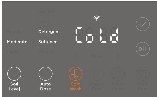
1. Press and hold **COLD WASH**
