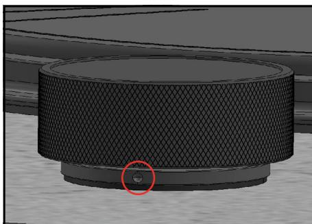
11. When placing the knobs in the worktop, **note the markings**. These indicate the front (Top Side) and the top (Front Side) of the knob.
