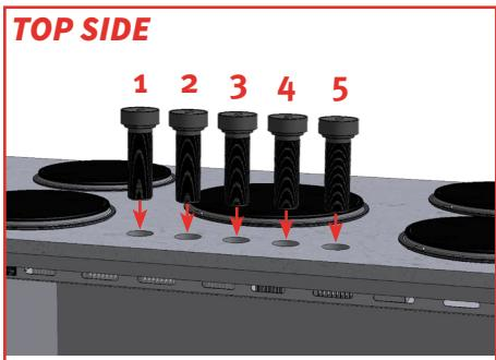
10a. In the case of a Top Side **PITT® Cooking unit**, place the knobs in the recesses at the top of the countertop. **Note the numbering.**
