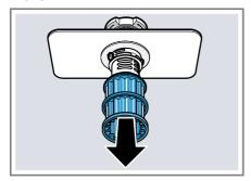
4. Press the locking catches 10 together and lift the coarse filter out ②.
